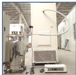
LN 2 /CO 2 backup system
